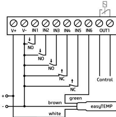
*In our example IN1, IN2 and IN3 inputs are normally open (NO), IN4 and IN5 inputs are normally closed (NC), while IN6 input is a temperature sensor (easyTemp).*
