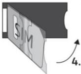
4-5. Fold down the socket and pull back the slider to its original position until you hear the click.
