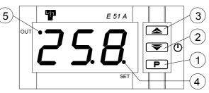
1 - Key P : Used for setting the Set point (press and release) and This document is the exclusive property of TECNOLOGIC for programming the function parameters (hold pressed for 5 sec.) and confirm the values.
