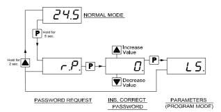
Note: If the Password gets lost, just cut off the supply, push P key and keeping it pressed for 5 seconds whilst switching on the supply to the instrument.
