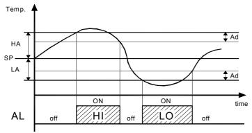
The maximum and minimum temperature alarms can be disabled by setting the relative parameters "HA" and "LA" = oF.
