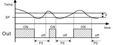
Third control (par. "P3") foresees an inhibition to the activation of 4.6 - KEYBOARD LOCK FUNCTION the output "Out" by a time delay that starts when the output was On the instrument it's possibile to lock completely the keyboard. turning on last time (delay between switching-on).
