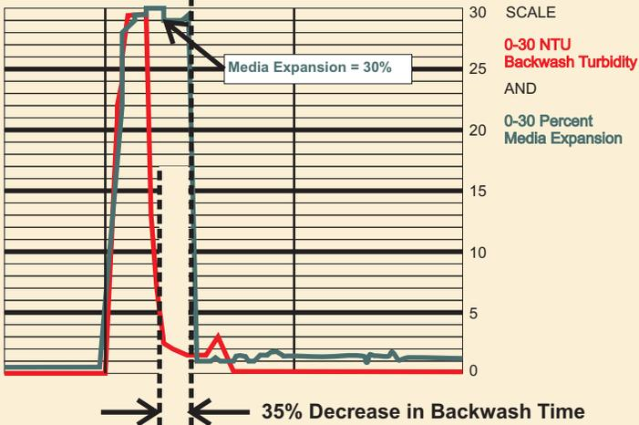
**Backwashing based on time may not expand the media properly, leading to formation of mud balls and mud cracks and reducing efficiency. EchoSmart washing ensures proper fluidation and cleaning of the filter media every time. Plus, turbidity monitoring with the same smart sensor allows you to end the backwash as soon as the wash water is clean. One customer reduced their backwash time by 35%!**
