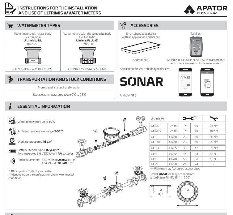
COMPONENTS REQUIRED TO INSTALL WATER METERS
