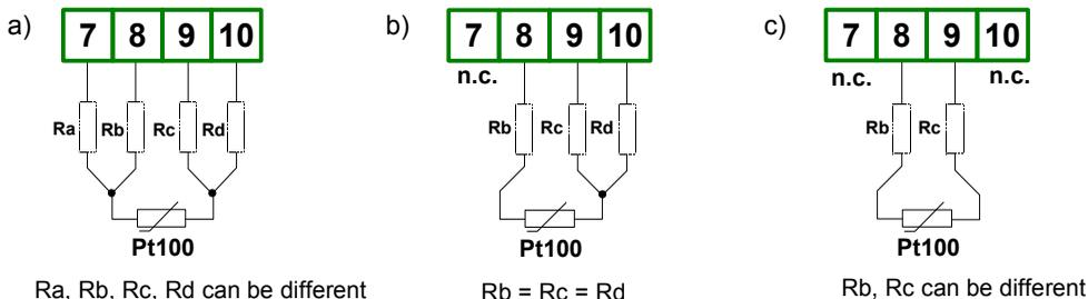
Figure. 4.7. Connection of sensors:
