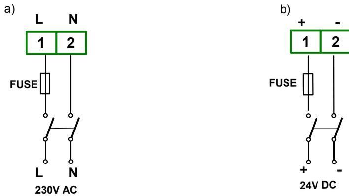
Figure 4.6. Connection of power supply
