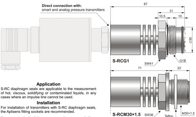
Recommended minimum measuring range 0.4bar (for pressure transmitters)
