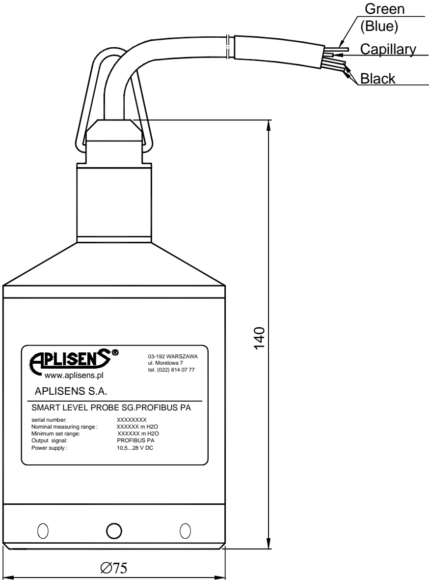
Fig.16. Smart level probe SG.Profibus PA - dimensions.
