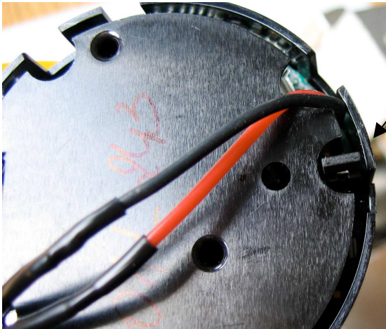
Fig. 4a. Back lighting jumper view at transmitter electric board (unit display back side).
