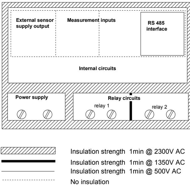
Fig. 3.1. Schematic diagram showing the insulation between individual circuits of the unit.
