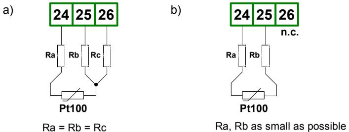
Fig. 4.9. Connection of Pt100 sensors for channel no 1:
