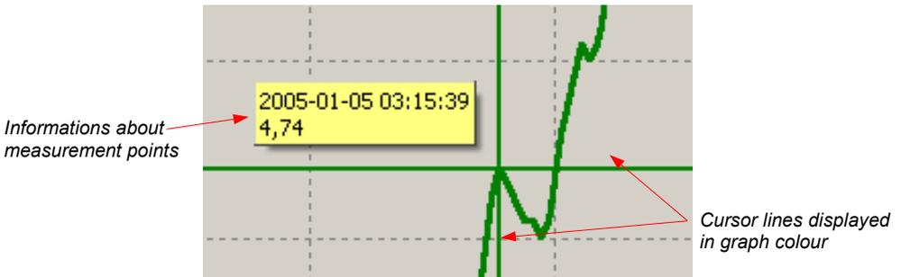
Fig. 3.9. Graph with special tracking cursor
