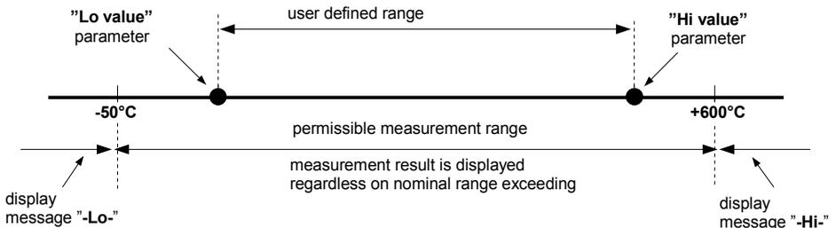
Fig. 6.1. Definition of measurement ranges
