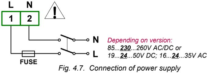
Fig. 4.7. Connection of power supply
