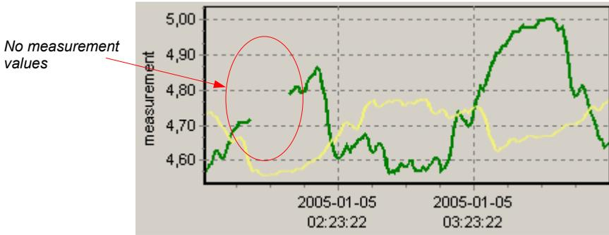
Fig. 3.10. Interruption in the graph (e.g. sensor fault)
