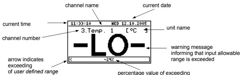
Fig. 6.10. Exceeding allowable range in "Single channel" mode
