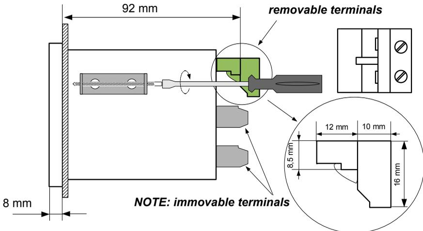
Fig. 4.2. Installing of brackets, and dimensions of connectors.
