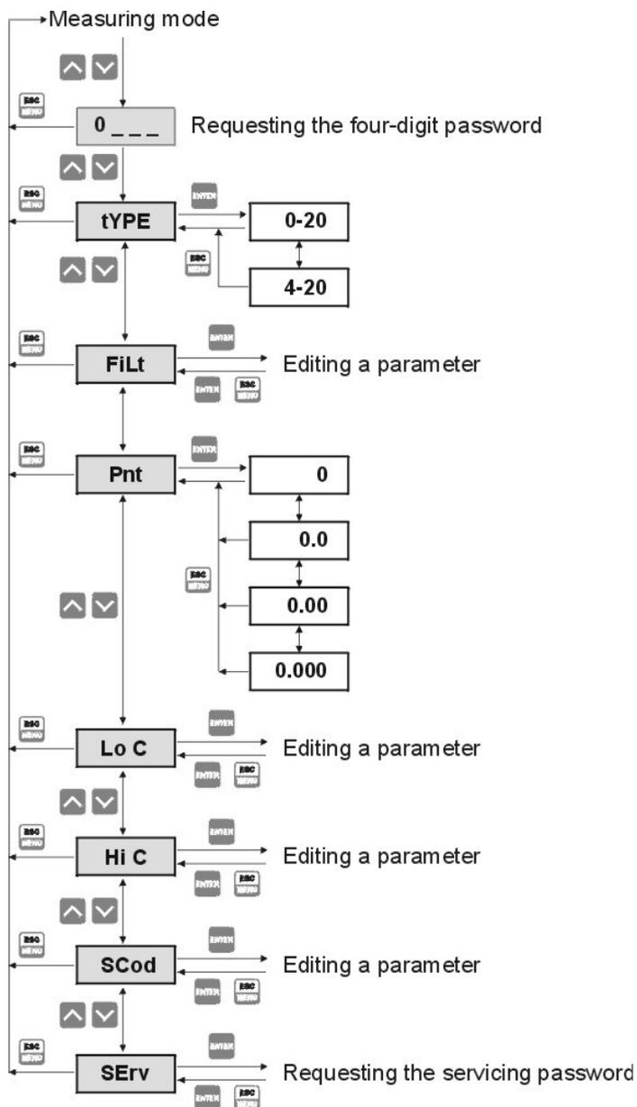
Fig. 3 Structure of the programming menu
