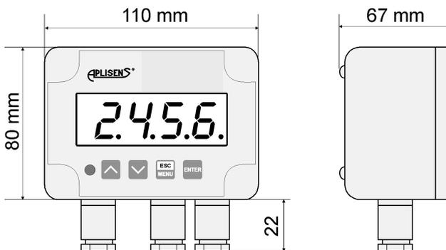
Fig 1 External dimensions of the measuring instrument
