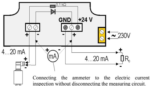
Fig. 2 Scheme of the electric leads
