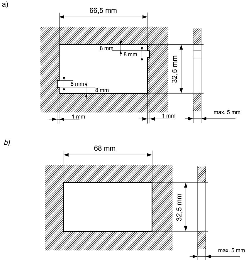
Figure 4.1. Mounting hole dimensions: a) recommended b) allowable
