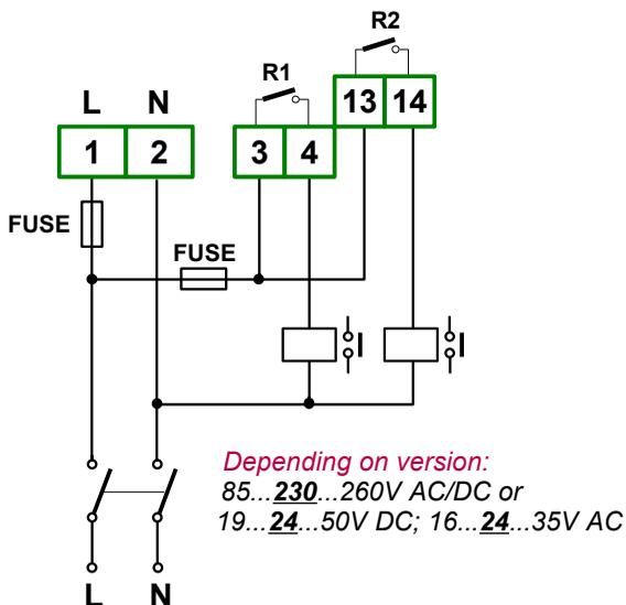
Figure 4.10. Connection of power supply and relays
