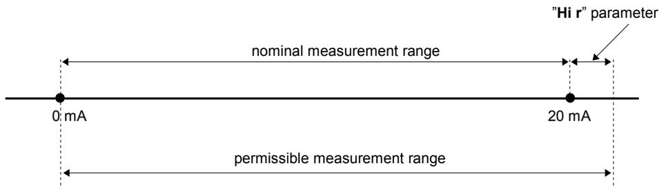
Figure 6.2. Definitions of measurement ranges in mode 0 ÷ 20mA
