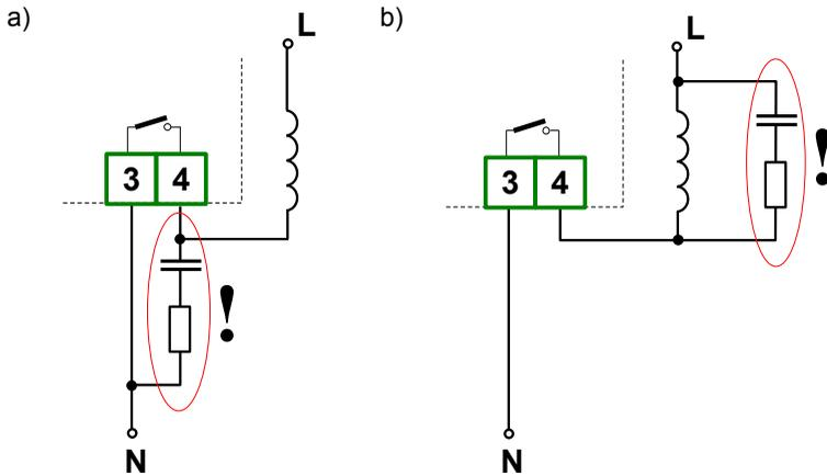
Figure 4.11. Examples of suppression circuit connection:
