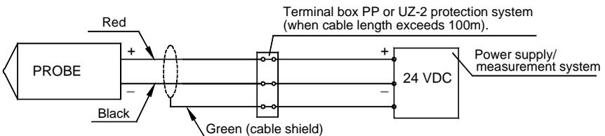
Figure 3B. Connection of SGE-25, SGE-16, SGE-25S and SG-25C in a two-wire system (4...20mA output signal). Not applicable to Ex version.
