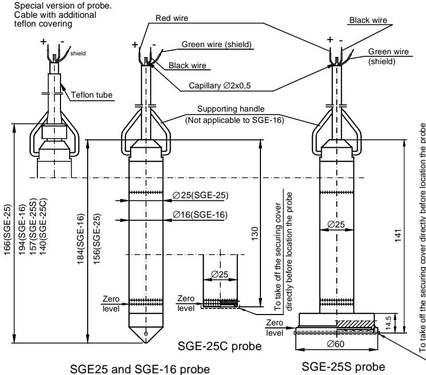
Figure 3. SGE-25, SGE-16, SGE-25C and SGE-25S probes – dimensions
