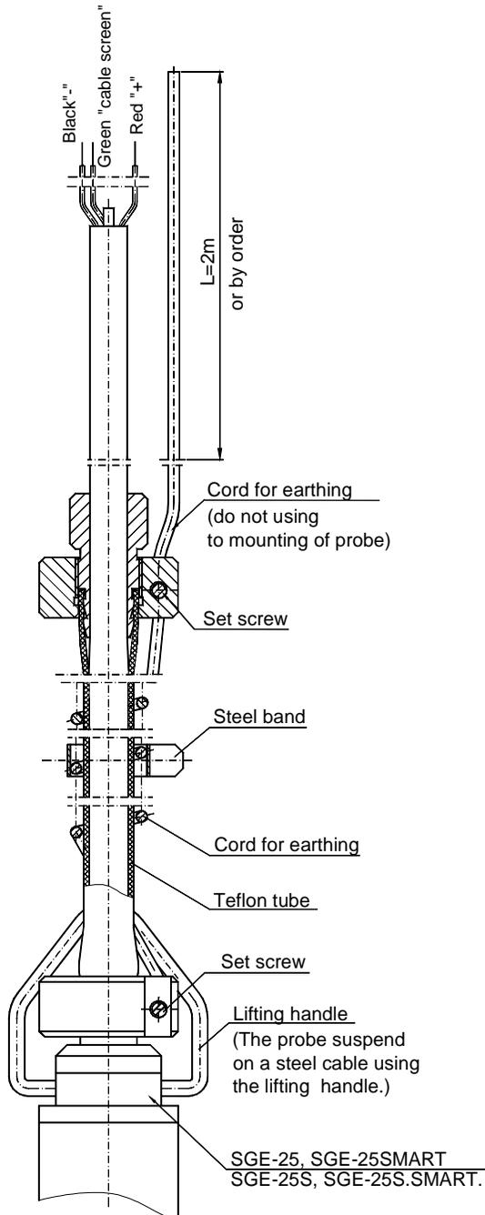
Figure 4. The probe in Ex-version with a cable with a Teflon shield.
