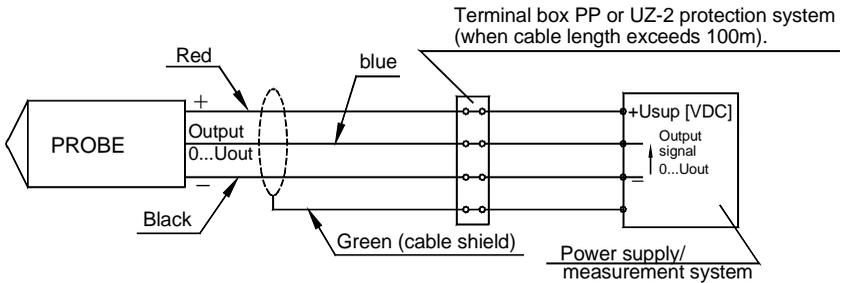
Figure 3A. Connection of SGE-25, SGE-25S and SGE-25C in a three-wire system (0...10V output signal). Not applicable to Ex version.
