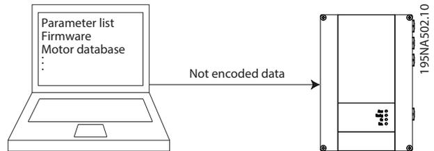
Illustration 2.9 Data Transfer from PC to Frequency Converter
