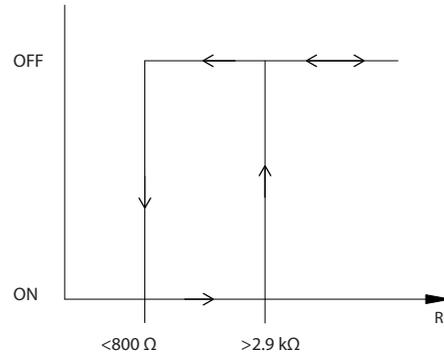
Illustration 3.7 Frequency Converter Operation with Thermistor
