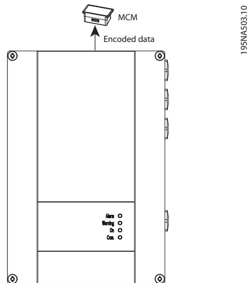
Illustration 2.10 Data Transfer from Frequency Converter to Memory Module
