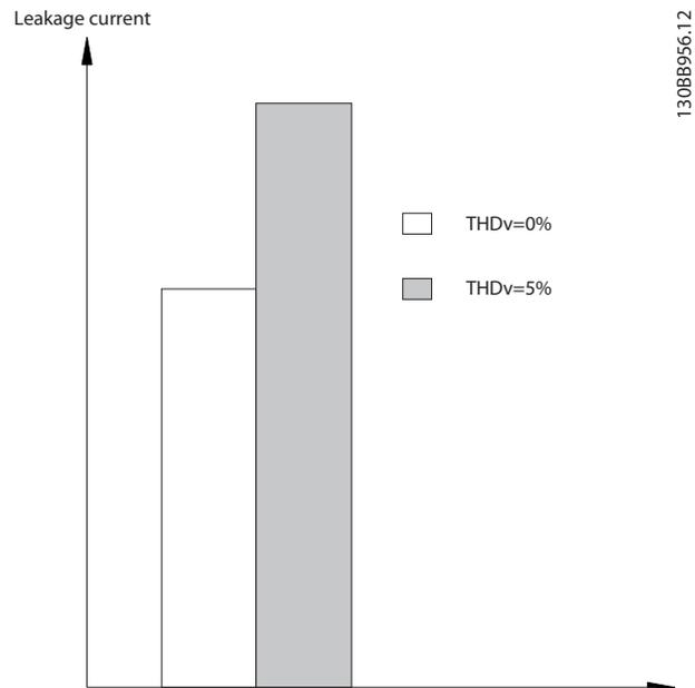
Illustration 2.22 Line Distortion Influences Leakage Current
