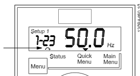
Illustration 7.7 Indicating Motor Direction
