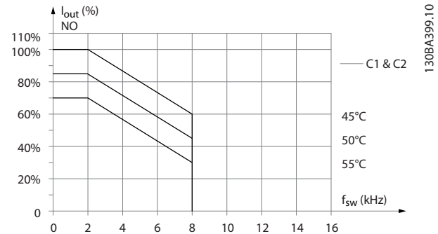
Illustration 5.16 Derating of I_{out} for Different T_{AMB, MAX} for Enclosure Sizes C1 and C2, using SFAVM in Normal Overload Mode (110% Overtorque)
