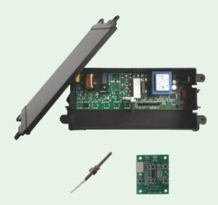
FEGR018 is an electronic system for the hoods oven management and is able to control a single phase induction motor of 350 W, a solenoid valve and, thanks to the keyboard provided in the supply, also the suction system's lights. The device requires that the user, through the keyboard commands, turn on and off the suction motor: when the motor is turn on the maximum speed activation is automatic and, in particular, slaved to the
