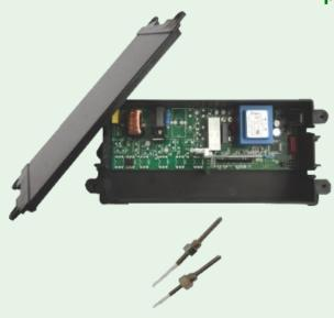
**FEGF01** is a microprocessor system designed to control the suction motor of an oven hood **without** the **operator intervention**. The device is able to turn on and turn off independently the motor and to set two different speeds: the first, which provides a reduced air flow, and the second that realizes the maximum air flow.
