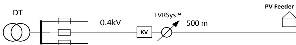
Figure 9-13 Example grid branch with 500 m cable section
