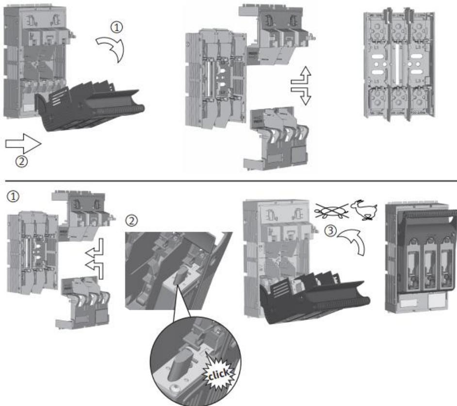
Figure 8-8 Operation fuse switch disconnectors
