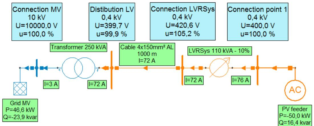
Figure 7-9 Low voltage grid with voltage boost along the cable regulated through LVRs
