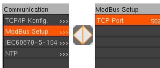
Figure 10-32 Modbus Setup
