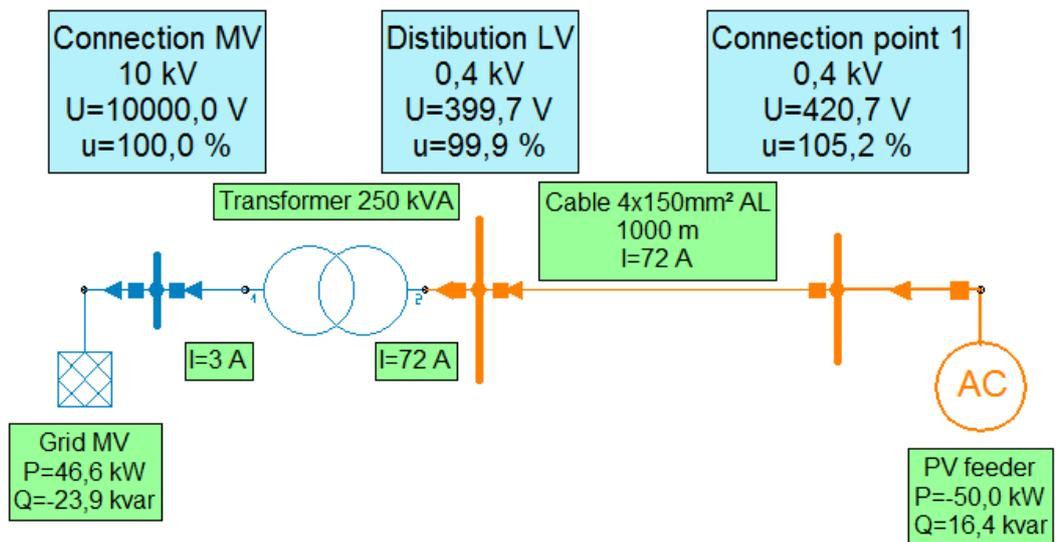
Figure 7-8 Low voltage grid with voltage boost along the cable (example)
