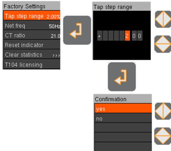
Figure 9-28 Setting the factory parameters
