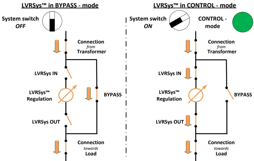
Figure 8-3 Circuit principle Bypass and operation
