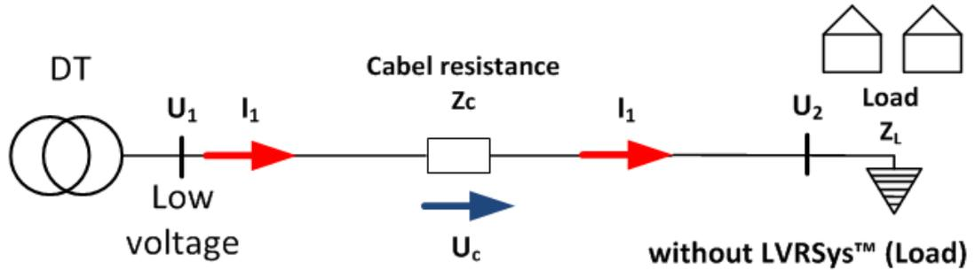
Figure 7-4 Low voltage grid with voltage drop along the cable
