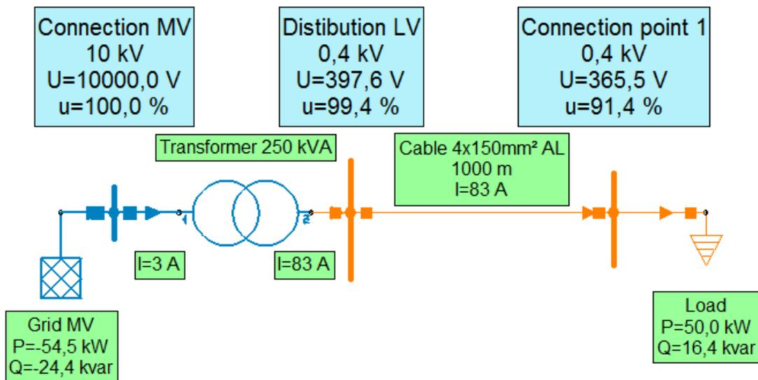
Figure 7-5 Low voltage grid with voltage drop along the cable (example)
