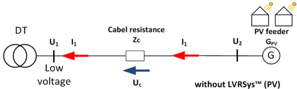
Figure 7-7 Low voltage grid with voltage boost along the cable
