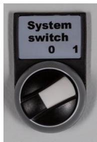
0 *Figure 9-3: System switch (system on)*
