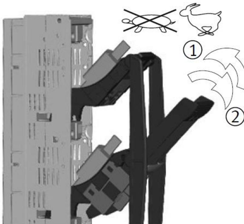
Figure 8-6 Operation switch disconnectors
