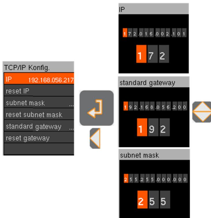
Figure 10-31 Overview of the TCP/IP configuration
