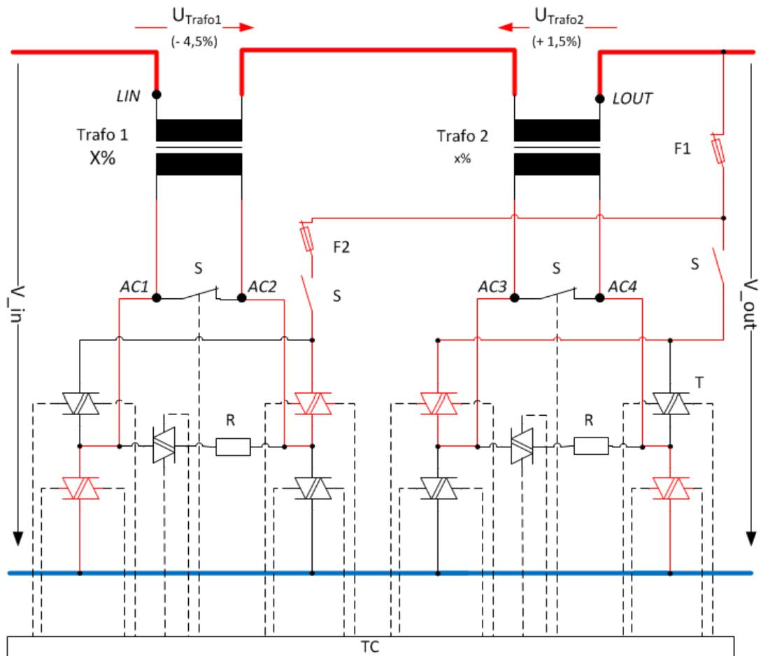
Figure 7-2 Example of 3% voltage reduction
