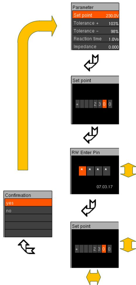
Figure 9-9 Setting the regulator parameters
