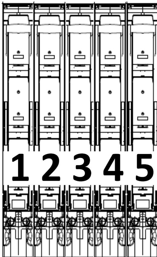
Figure 8-7 NH switch disconnectors
