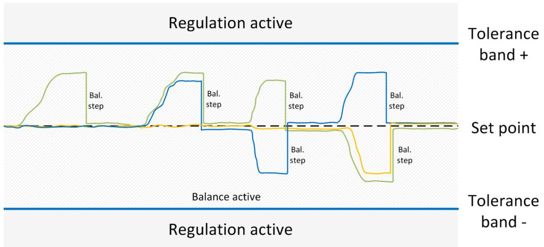
Figure 9-14 Example of unbalanced phase voltages
