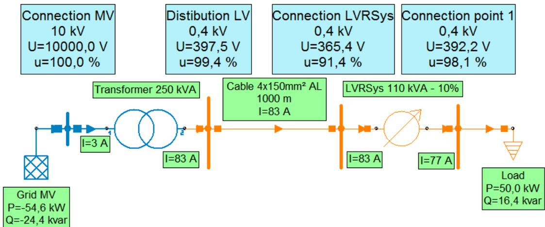
Figure 7-6 Low voltage grid with voltage drop along the cable regulated through LVRsSys
