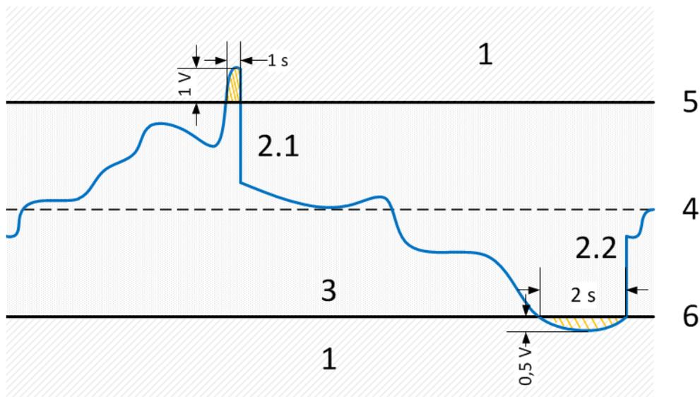
Figure 9-11 Tolerance band zone reaction time
