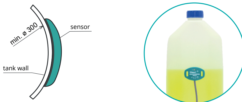
Fastening the FLD-32 using self-adhesive layer
