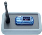
The data logger, which operates within the 868 MHz (EU version) or 915 MHz (US version) ISM frequency band, receives and stores the measured data from up to ten MSR385SM transmitter modules. Flash memory for data security in the event of a power failure. Brilliant, high-contrast OLED colour display.
