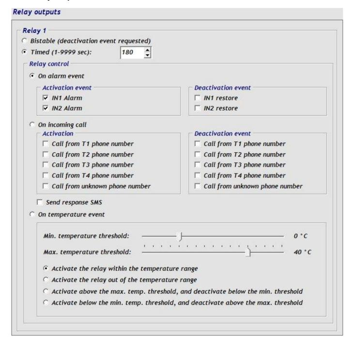
The module has 2 normally open relay outputs which can be controlled by events, by incoming call or by temperature events.
