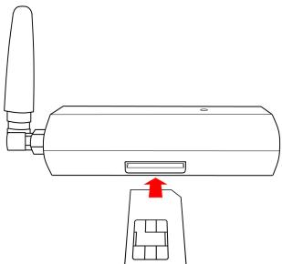
Removing the SIM card: push the overhanging part of the SIM card towards the modem until it clicks, then release and pull out the card from the slot.
