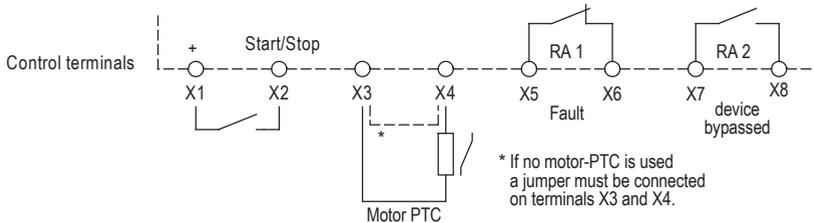
If the motor temperature exceeds the switching threshold, the motor PTC triggers a fault. The soft starter switches the motor off and is interlocked in fault mode. The fault is signaled by the yellow LED repeatedly flashing two times and by an opening of the relay contact between the terminals X5 and X6.
