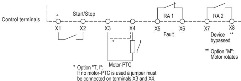
The input resistance of the control inputs is ca. 10kOhm. To control them, it is necessary to use switching contacts enabling reliable switching of the lower control currents (e.g., AgNi+Au)!
