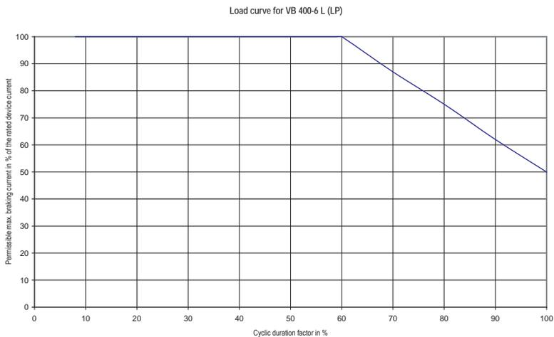
$$\text{Cyclic duration factor (r.c.d.f.)} = \frac{t_B}{\text{Cycle time}} \times 100$$
