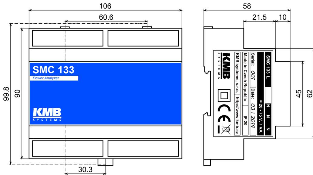
Figure 2: Dimensions of the SMC 133 analyzer.
