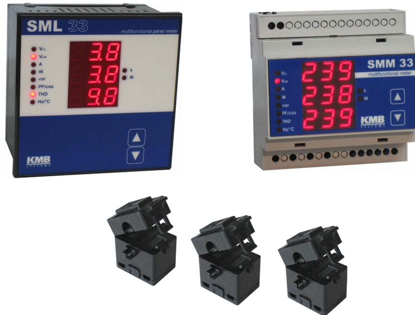
The instruments are designed to measure and monitor line and phase voltages, currents, active and reactive power, power factors, THD as well as frequency in single-phase and three-phase low voltage, high voltage, and very high voltage power systems. They further allow informative measurement of temperatures within a switchboard cabinet using an inbuilt temperature sensor.
