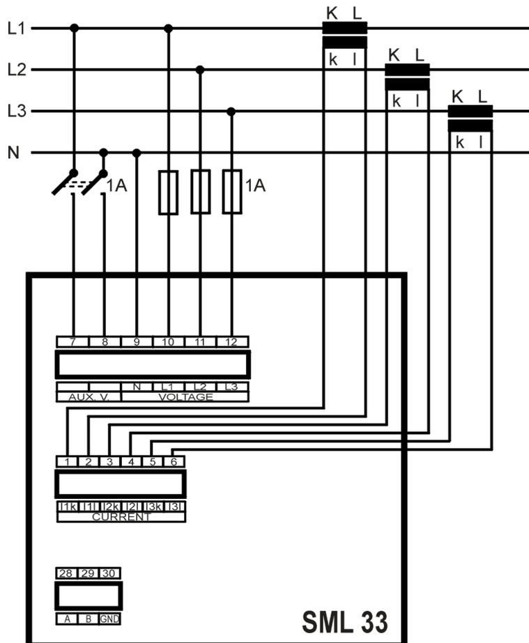
*SMM33 U 230 X/5A Wiring Diagram*
