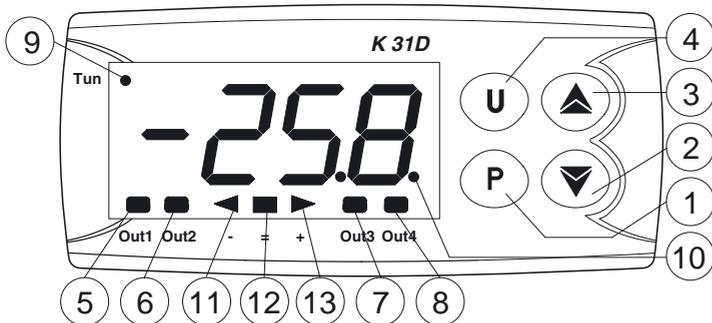
**1 - Key P:** This is used to access the programming parameters and to confirm selection.
