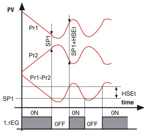
Example of differential ON/OFF control (On.FA) with "Func"= Cool
