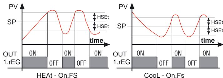
The control works in the following way: in the case of reverse action, or heating ("Func"=HEAt), it deactivates the output, when the process value reaches [SP + HSEt] in case of symmetrical hysteresis, or [SP] in case of asymmetrical hysteresis and is then activated again when the process value goes below value [SP - HSEt].
