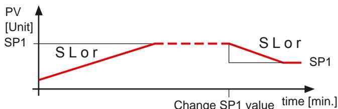
If it is desired an automatic cycle from the power ON instead it is necessary to program the par. “nSP” = 2, to program the two Set Point values “SP1” and “SP2” and naturally to program the par. “SLor”, “dur.t” and “SLoF” with the desired values.
