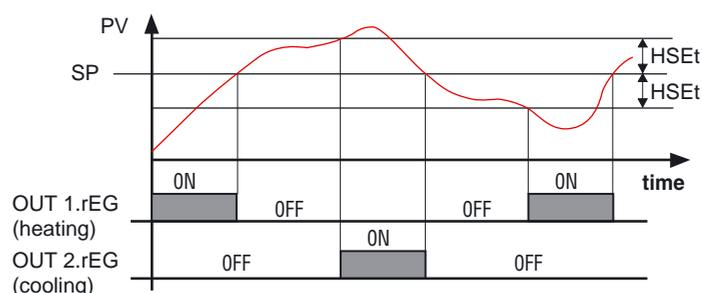
If 2.rEG output is used to control compressor is possible to use the "Compressor Protection" function that has the meaning to avoid compressor "short cycles".
