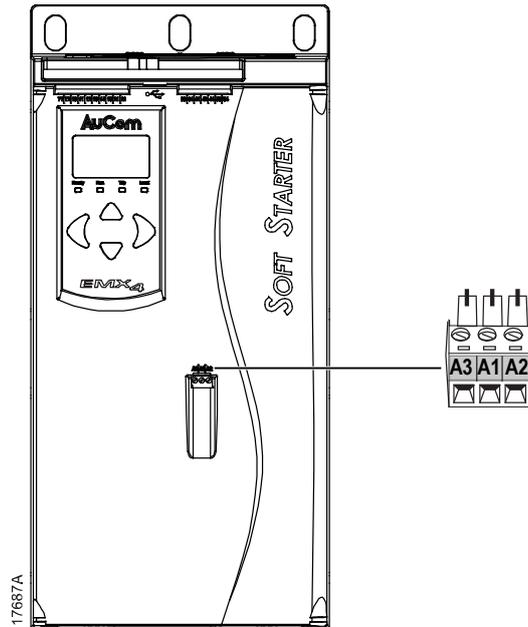
Connect the control supply according to the supply voltage being used:
