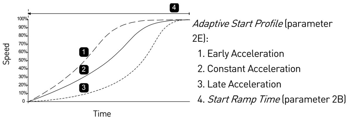
If replacing a motor connected to an EMX4i programmed for Adaptive Control starting or stopping, the starter will need to learn the characteristics of the new motor. Change the value of parameter 1B *Motor Full Load Current* or parameter 2L *Adaptive Control Gain* to initiate the re-learning process. The next start will use constant current and the next stop will use timed voltage ramp.
