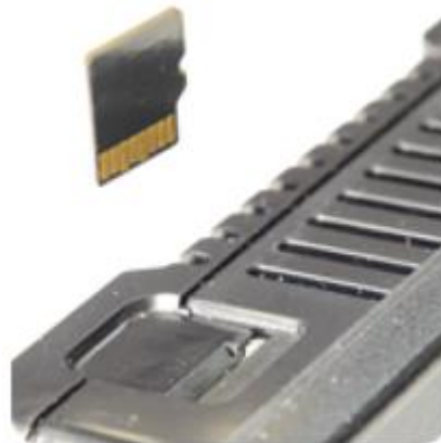
Figure 10.2 - Installing Removable Memory Card
