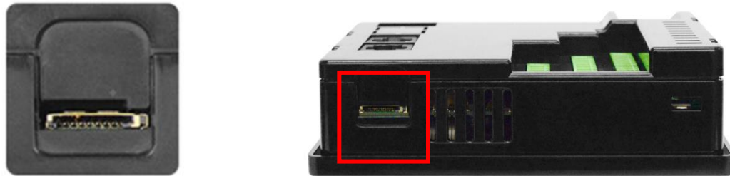
Figure 10.1 - Removable microSD Memory Card Slot
