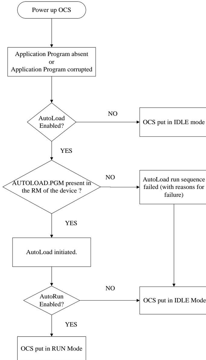
Figure 16.8 – Flow Chart for AutoLoad
