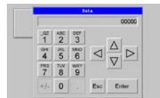
In addition, to edit a single numeric digit, use the ← or → key to select the digit and then either press a numeric key or use ↓ or ↑ to modify the digit. In any case, after entering the new desired value, press the **Enter** key to save it; otherwise press the **ESC** key to cancel the edit.
