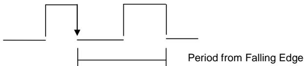
Figures 11.3-11.4 – Period Measurement, Rising Edges & Falling Edges
