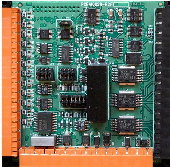
Figure 10.2 – EXL6 I/O Cover Removed (sample I/O board)
