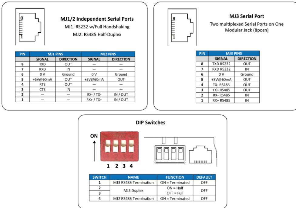
Figure 5.1 – Wiring & Dip Switches
