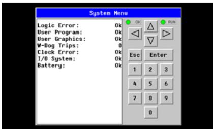
The View Diags Sub-Menu displays up to 11 System Diagnostics, none of which are editable.
