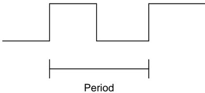
Figures 11.6 & 11.7 – PWM, two parameters, Duty Cycle & Frequency
