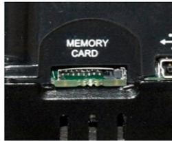
Figure 9.1 – Removable MicroSD Memory Card Slot
