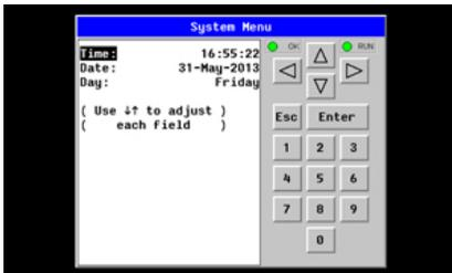
The Set Time/Date Sub-Menu displays three System Settings. **Time** and **Date** may be edited, and **Day** is automatically calculated from the **Date** setting. Note that **Time** and **Date** are split into three fields each, all of which may be edited. Use ← or → to select a field and then use ↓ or ↑ to edit the field.
