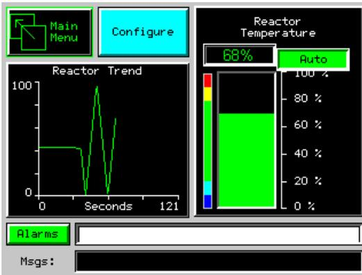
Figure 13.3 – Typical Screen Jump Object
