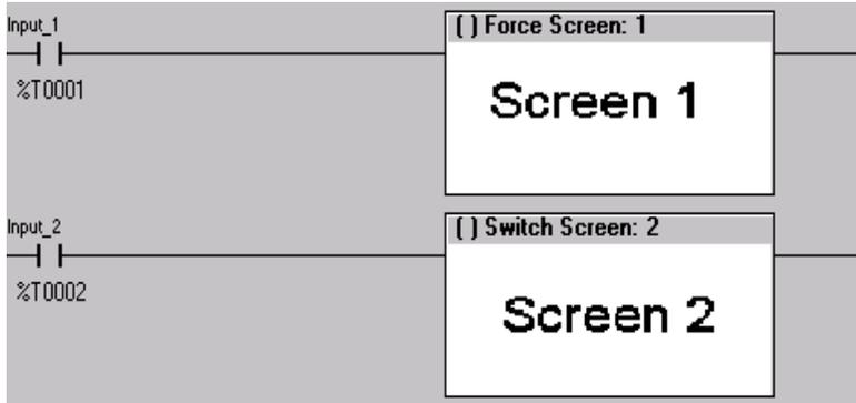
Figure 13.4 – Force and Switch Coils in Ladder Programming
