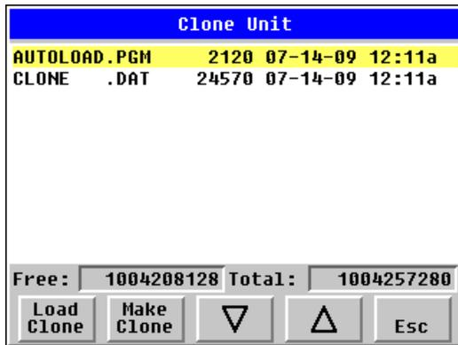
Figure 17.4 – Clone Unit Files
