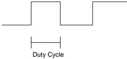
**Frequency** - The Frequency is a 32 bit value indicating the output frequency in Hertz. One over the frequency is the period.
