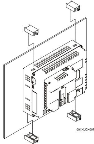
Figure 3.2 – EXL6 OCS with Mounting Clips
