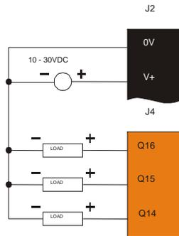
Figure 10.4 – Typical Output Wiring
