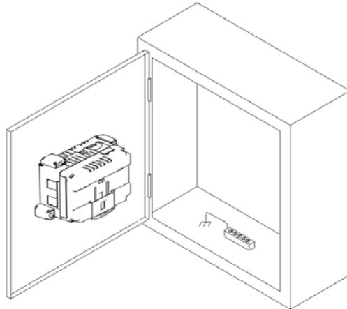
Figure 3.1 – Panel Mounting of an EXL6 Series OCS
