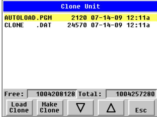
Figure 17.7 – Clone Unit Menu after Cloning
