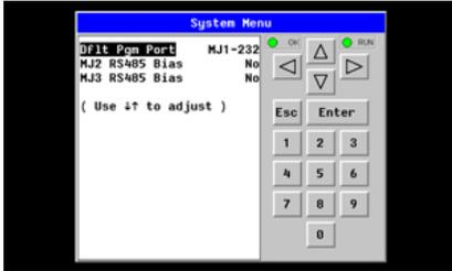
The Set Serial Ports Sub-Menu displays three System Settings, all of which may be edited, and one optional item. For the **Dflt Pgm Port** System setting, only MJ1-232 can be selected, unless a Modem (XMC) COM module is installed.
