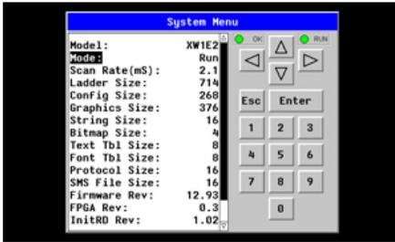
The View Status Sub-Menu displays up to 19 System Settings. Only the **OCS Mode** System Setting is editable.
