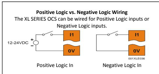
Figure 10.6 – Positive and Negative Inputs
