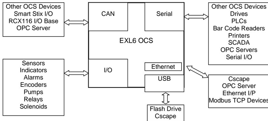
Figure 2.2 – Visual Overview of Types of Devices that can be connected to EXL6 OCS
