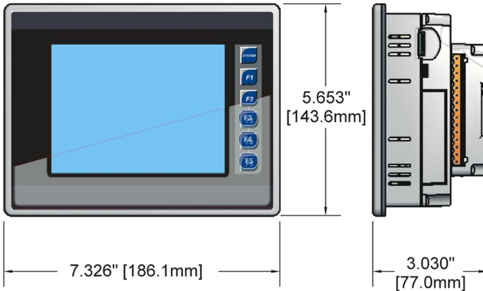
Figure 3.5 – EXL6 OCS Dimensions
