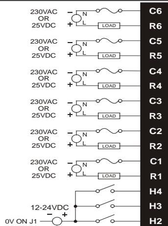
Figure 10.5 – Relay Fusing
