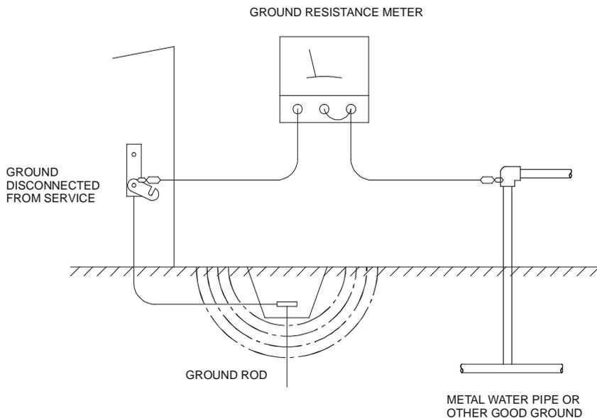
Figure 4.1 – Two-Point Ground Connection Test
