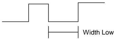
Figures 11.1-11.2 - Pulse Width Measurements, High & Low
