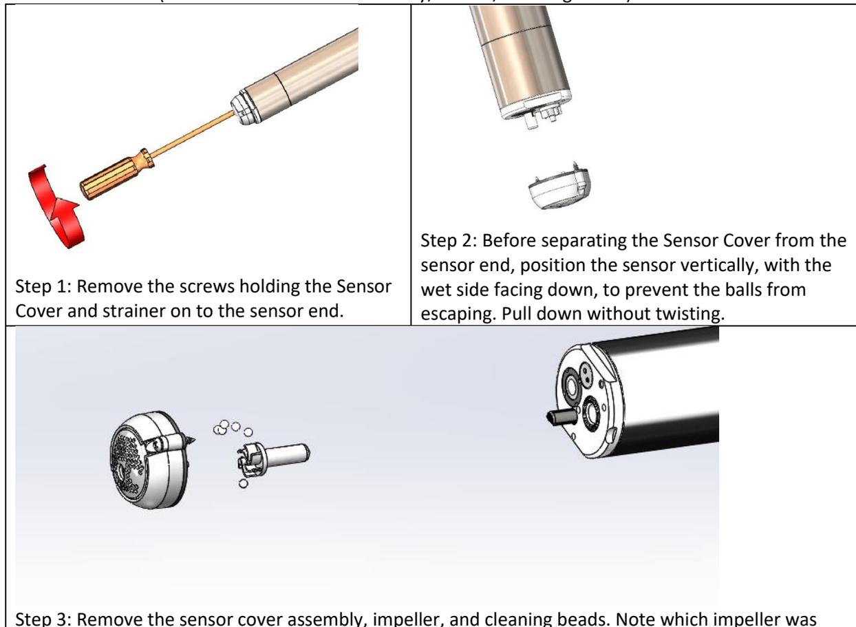
installed (Large Pin or Small Pin). Then discard those parts. If the impeller has a small pin, then proceed to Step 4. For large pin impeller, skip ahead to Step 6 since the large pin bearing does not require replacement.
