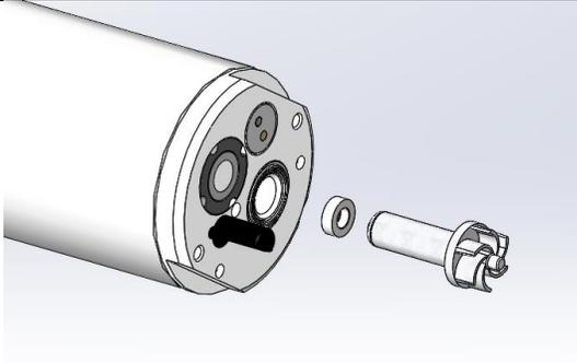
Step 6: Install new impeller and bearing for small pin impeller. For large pin impeller, replace only the impeller.
