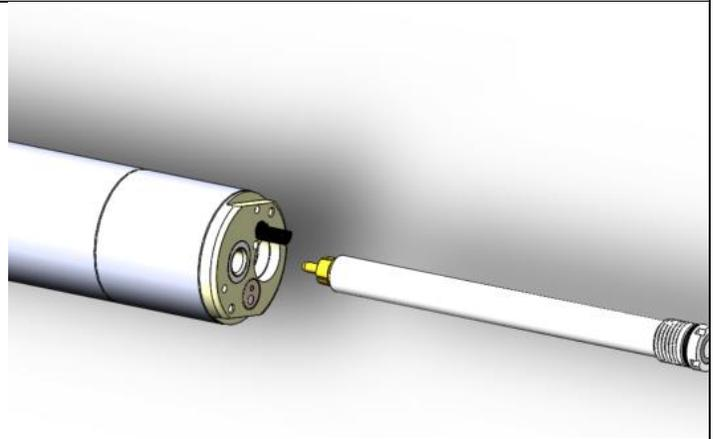
*Figure 19: Remove the pH Sensor and discard. Replace with a new one. Make hole is wiped clean. Replacement sensor has silicone grease and an o-ring applied.*
