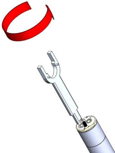
*Figure 18: Unthread the sensor by twisting counterclockwise (CCW).*
