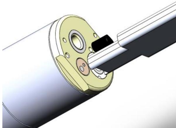
*Figure 17: Insert prongs flush with pH Sensor.*
