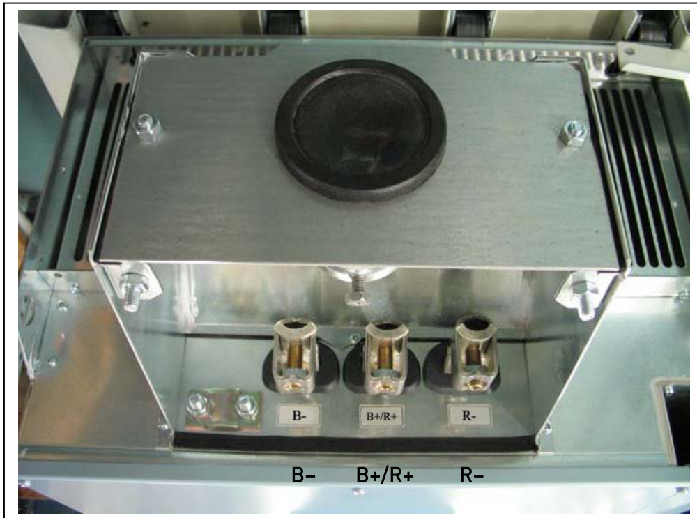
Figure 6-22. DC and brake resistor terminals on FR9; DC terminals marked with B- and B+, brake resistor terminals marked with R+ and R-
