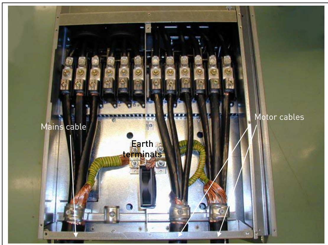
Figure 6-21. Cable installation in Vacon NXS/P, FR9
