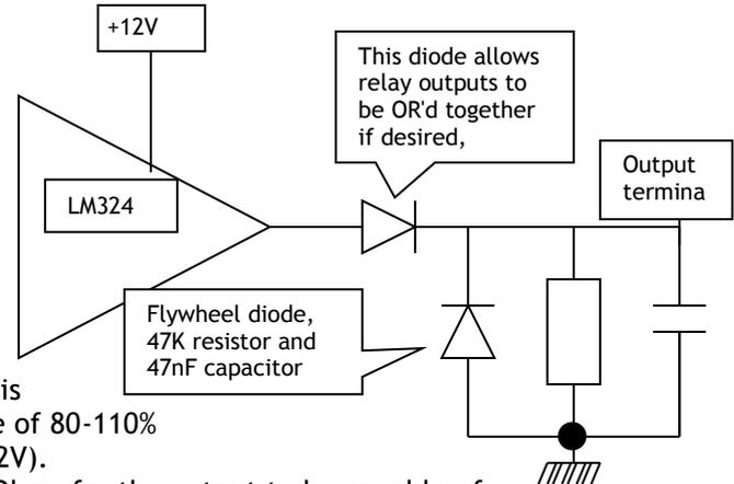
When driving relays, ensure the coil operating range is suitable. E. g. a 12V relay with a coil operating range of 80-110% will energise at voltages of 9.6V and above (80% of 12V).
