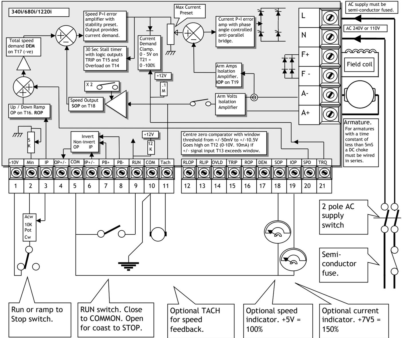
The +10V ref is connected to the speed pot by a switch giving a ramp to zero when opened.
