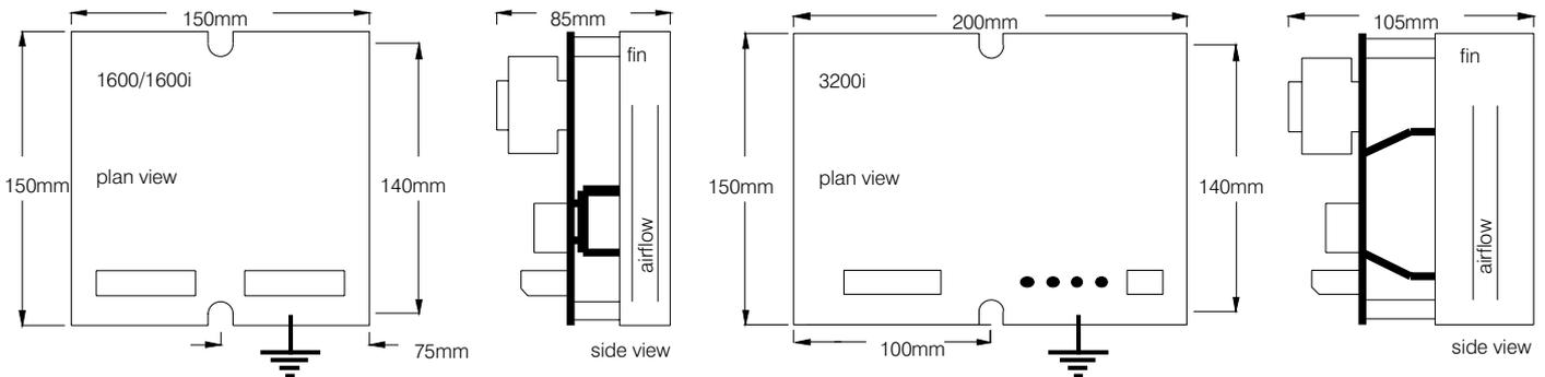
The unit should have a substantial earth connected to the heatsink earth screw provided. Employ a star washer adjacent to the heatsink for optimum earth continuity. The fixing bolts should be 5mm by 35mm for the 1600/1600i and 5mm by 50mm for the 3200 series.
