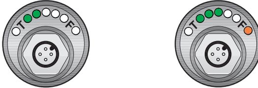
*Example: if the flow rate switching point is set to the 3rd LED, then the flow rate output switches (in the case of setting O) when at least such a flow rate is achieved, which lights the 3rd LED on the bar graph.*
