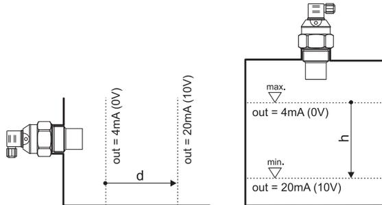
Fig. 19: Inverse mode (distance measurement)
