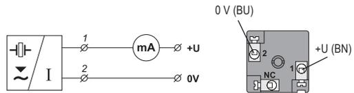
Fig. 15: Level meter connection diagram ("I" version) and the inside of the connector socket
