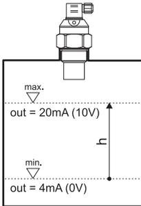
Fig. 18: Basic mode (measurement of level height)
