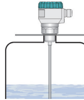
Fig. 7: Incorrect welding flange mounting to the tank
