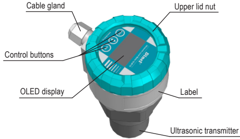
Fig. 16: Full view of ultrasonic level meter
