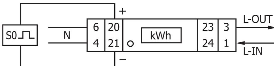
*When connecting the meter through a serial converter (RS485) for testing, please be aware that because of not implementing the complete Modbus infrastructure, there will be a need to put an additional resistor (120 ohms/ 0.25 watts) across the terminals (23 & 24) on the meter side.*
