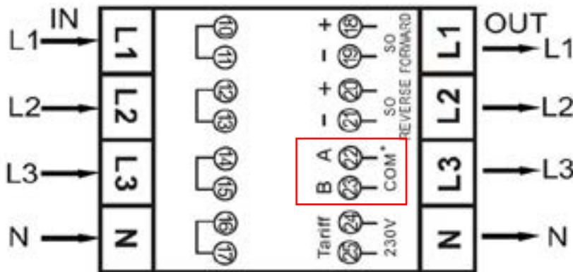
*When connecting the meter through a serial converter (RS485) for testing, please be aware that because of not implementing the complete Modbus infrastructure, there will be a need to put an additional resistor (120 ohms/ 0,25 watts) across the terminals (22 & 23) on the meter side.*
